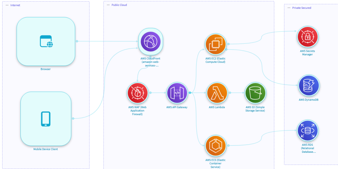
Figure 4: Topology proposed for the system architecture, designed using the IriusRisk tool
