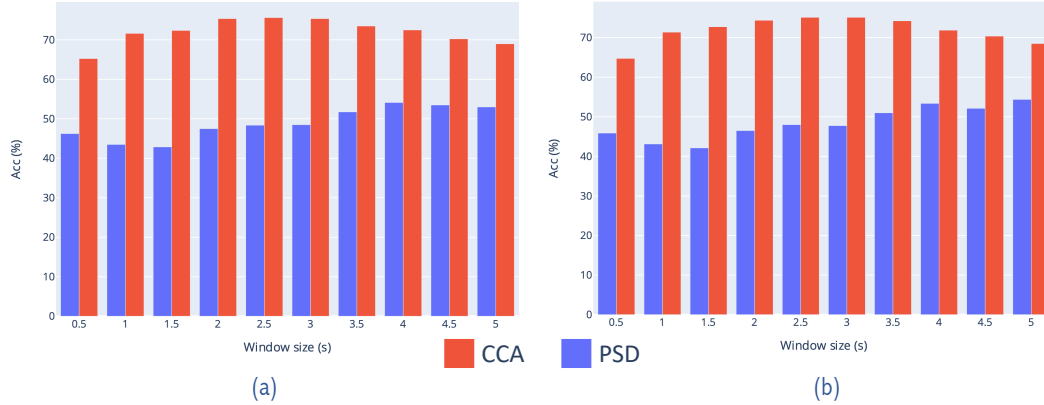
Figure 4.6: Average system accuracy using different time windows. In (a) the preprocessing without the eye blink subtraction algorithm. In (b) preprocessing with eye blink subtraction stage
