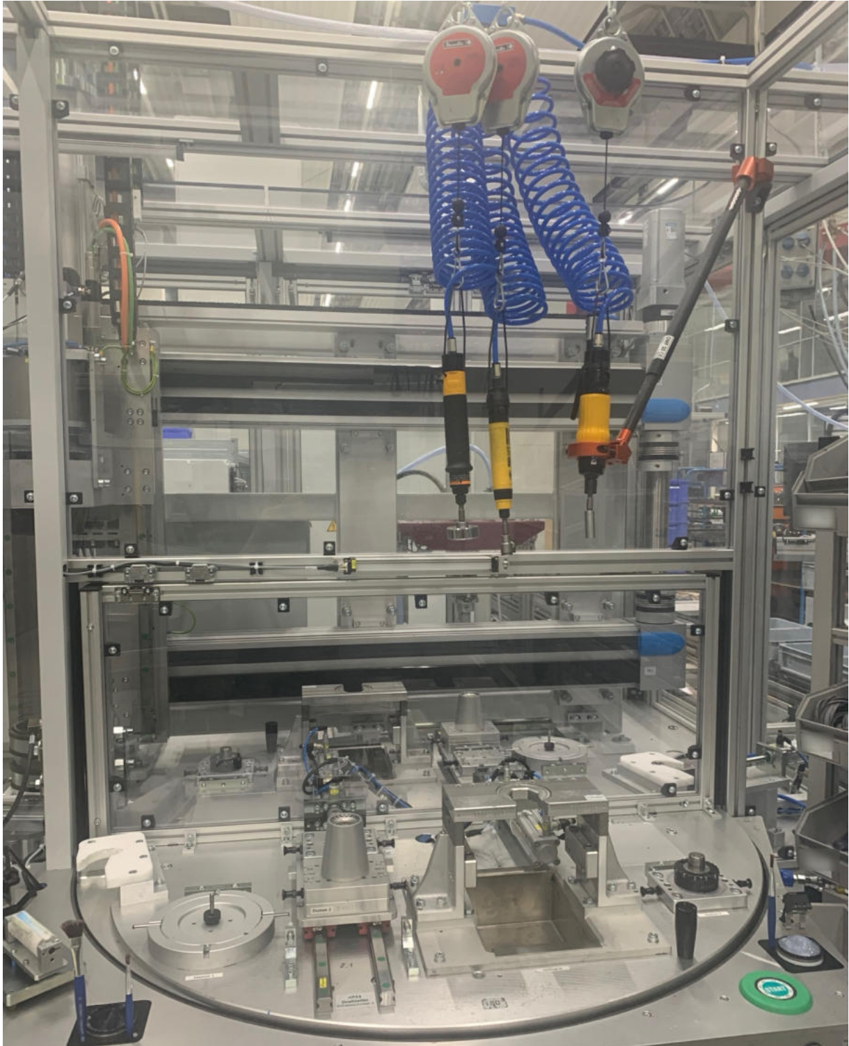
Figure 3 Assembly station 2 “Turntable”: Insert parts, start, insert new parts from the box coming through the assembly line
