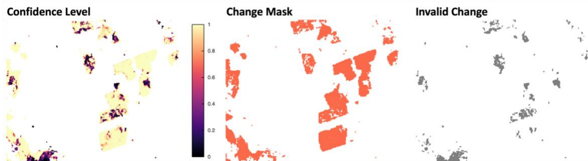
Figure 14. Confidence level and derived masks after bootstrapping the process of change point detection. Left: Confidence Level. Center: Valid change points (red). Right: Invalid change points (gray).
