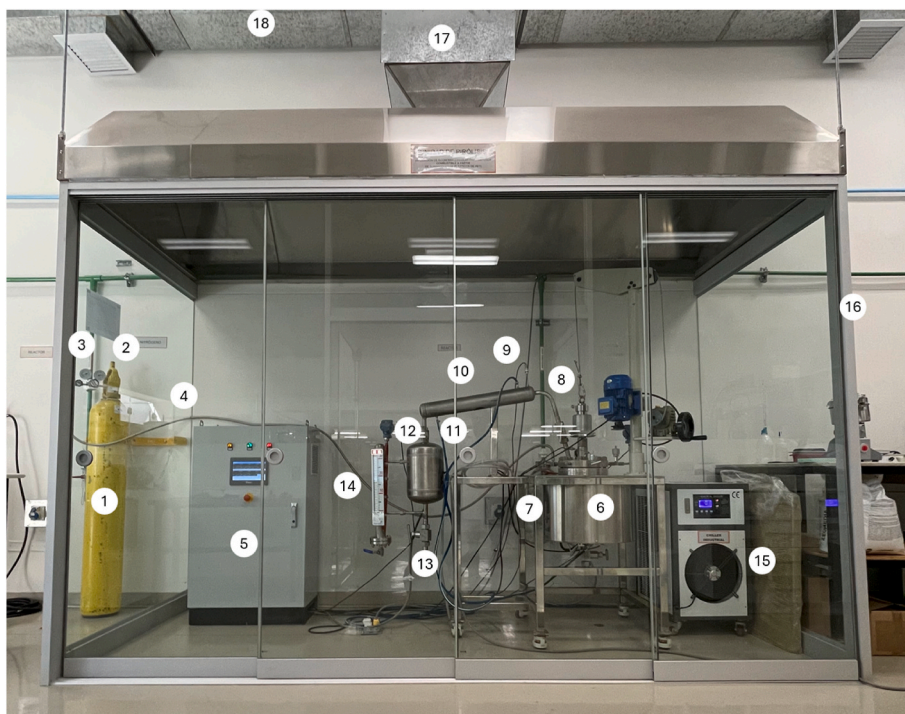
Fig. 2. Laboratory-scale fast catalytic pyrolysis unit with hermetic insulation and fugitive emissions treatment system.
