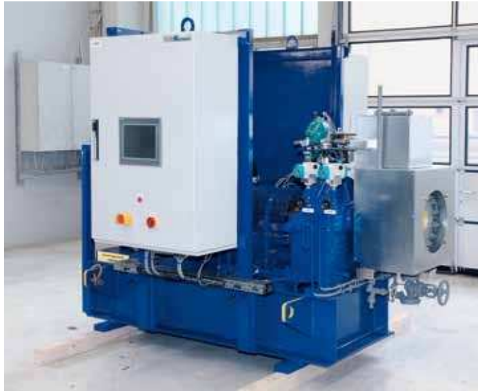
The control and operating unit with a 12-inch touch panel covers all necessary monitoring functions.
