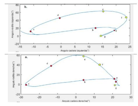
**Figure 7.** Cyclogram of transtibial prosthetic gait. Comparison of non-amputated leg (left leg) with the amputated (right) leg during transtibial gait, making use of cyclograms. a) loading response; b) mid-stance; c) terminal stance; d) pre-swing (*PSw*); e) initial swing; f) mid-swing; g) terminal swing
