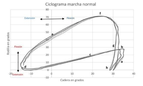
**Figure 6.** Cyclogram for analyzing gait. a) Initial contact; b) loading response; c) mid-stance; d) terminal stance; e) preswing; f) initial swing; g) mid-swing; h) terminal swing
