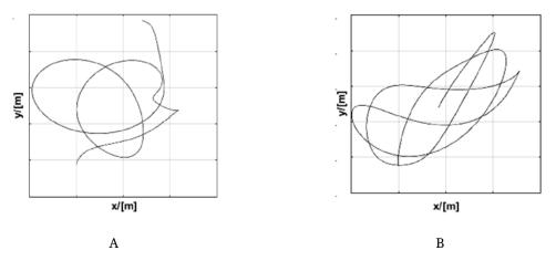
**Figure 8.** Trajectory described by the feet. A) Trajectory of the foot on non-amputated side. B) Trajectory of prosthetic foot. This indicates that more energy is required in the non-amputated foot to compensate for work not performed by the non-amputated foot
