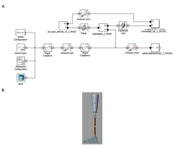
**Figure 2.** Diagram of representative shuttle locks of the prosthesis. A) Simulation of the prosthesis in Simulink®. B) Diagram of transtibial prosthesis obtained in Matlab® using 3D model developed using Solidworks®
