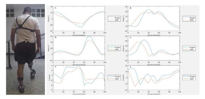
**Figure 10.** Angular trajectories for each articulation obtained through the model (red line) and laboratory study of gait (blue line). a) Right hip; b) Right knee; c) Right ankle; d) Left hip; e) Left knee; f) Left ankle
