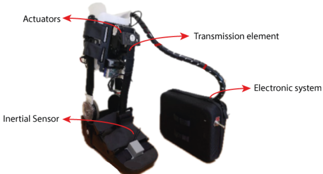
Figure 1.1: T-FLEX system. The figure illustrates the main components: the actuators that work in conjunction with the transmission elements to generate movement assistance, the electronic control system and the inertial sensor that detects the motion intention [13].
