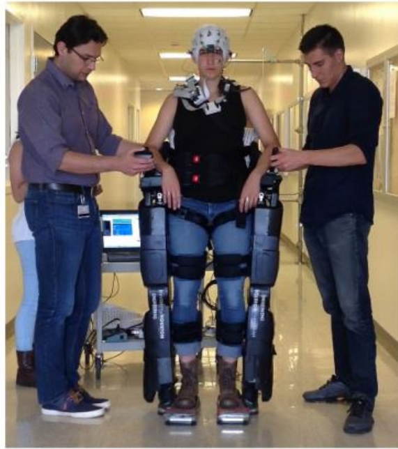
Figure 2.11: BCI system set up to control and evaluate REX device [87]
