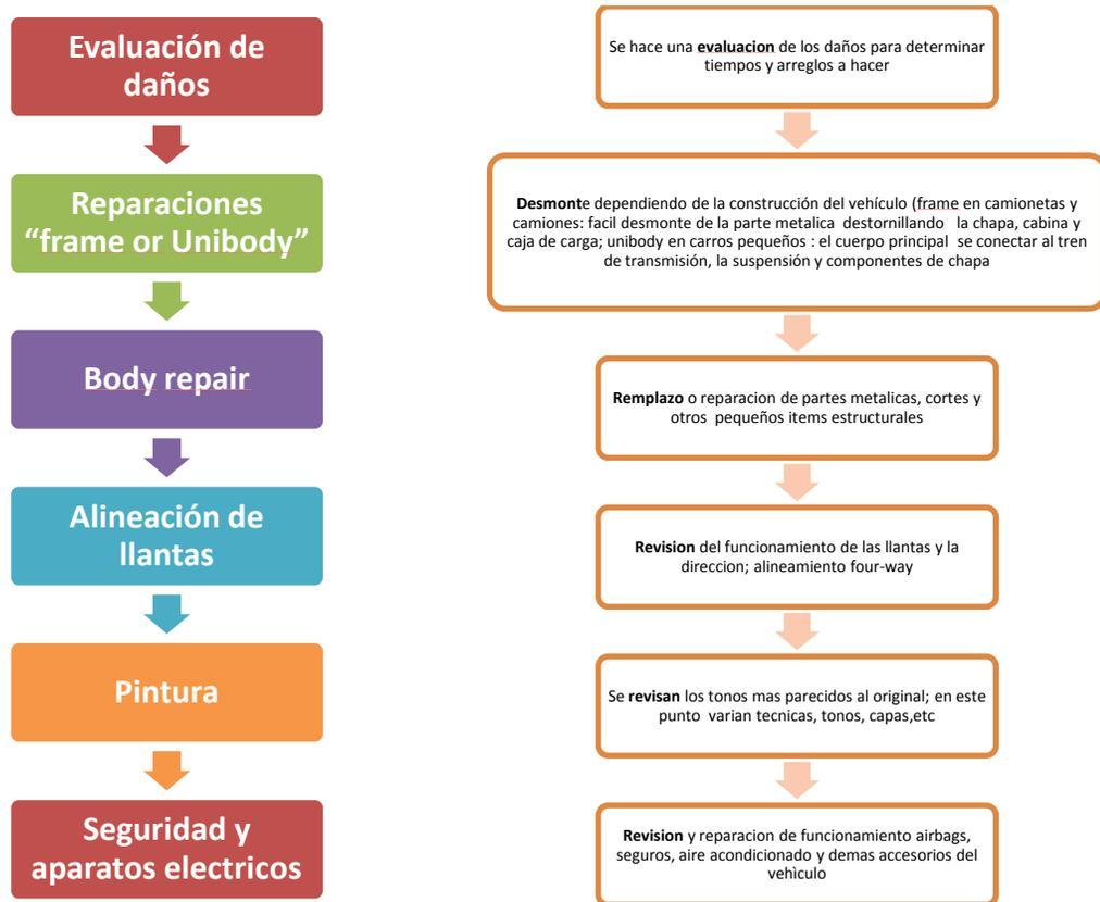
Ilustración 6: Ron's Auto Body and Paint Repair Process. Basada en contenido de <http://ronsautobodyandpaintvancouver.com/repair-process.php>, Heitzman body paint process <http://www.heitzmanbodyandpaint.com/services.htm>, Body and paint center of Hudson <http://bodyandpaintcenter.com/tomad>
