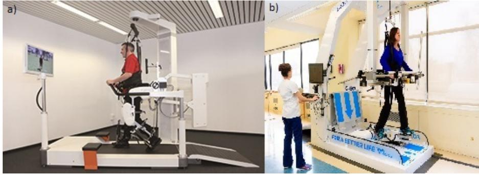
Figure 1.1: a) Lokomat system. A stationary system which influences on the patient's walking trajectory, rather than producing movements volitionally [15]. b) G-EO system. Robotic therapy aid for plegic or parietic limb movements that may help the functionality recovery recovery simulate gait and other more complex gait standards of gait such as the steps on stair [16], [13].
