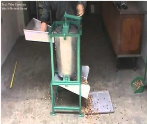
A green manual peeling machine with a hopper at the top and a collection tray at the bottom. It is shown in a kitchen or food processing area.                                                                    |
